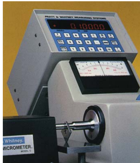
Mastering with a gage block
